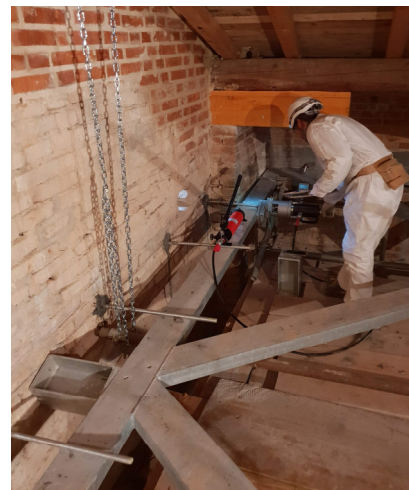
Figure 8: horizontal metal truss of the front façade Figure 9: Pull-out test on the connectors with the façade
