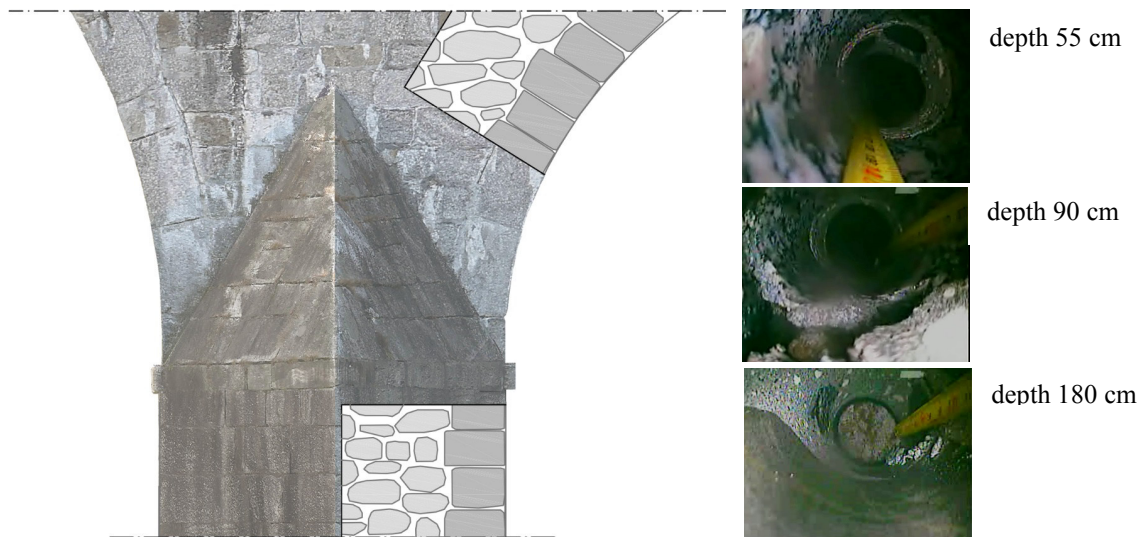
Fig. 4 a pile as shown in the Chapters; images coming from coring holes inspected with endoscopic video camera
