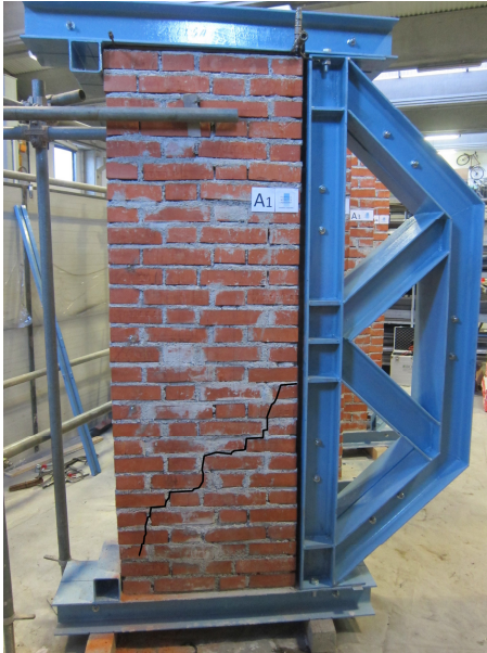
Fig. 4. Laboratory panels subjected to FJ-SCT: diagonal cracks are underlined - shear stress vs. horizontal displacement diagram
